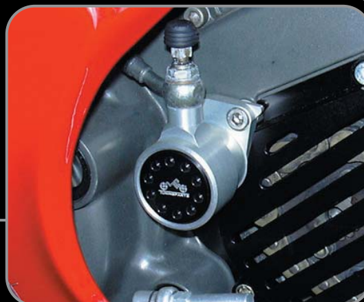
Aprilia clutch slave cylinder with mounting kit
