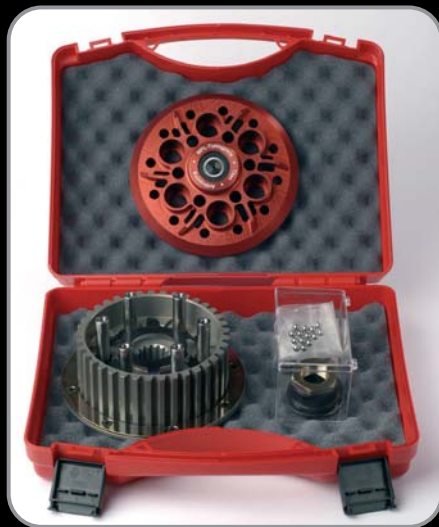
Pic.1: clutch with basket with inserts and open pressure plate
